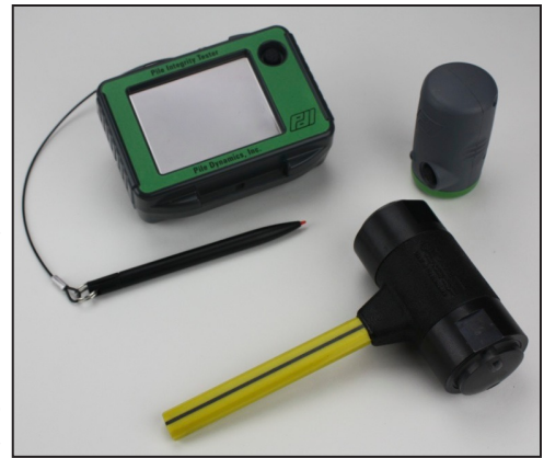
PIT-X with wireless accelerometer and handheld hammer.
